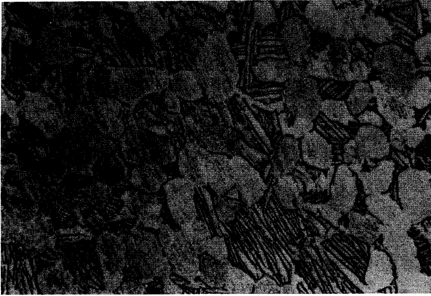
Fig. 1 Transverse section through specimen RAE1 923 cycles X 800 Etched — Kroll's reagent
