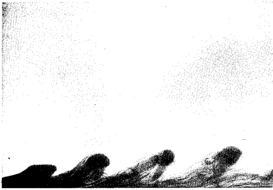
FIG. 4. Side view of hairpin vortices generated behind slot injector with pulsing rate 0.3 Hz, injection/free-stream velocity ratio, \zeta=0.325 , free-stream speed, u_\infty=2.5 cm/sec, and Reynolds number based on displacement boundary layer thickness, Re_\delta^*=208 .
