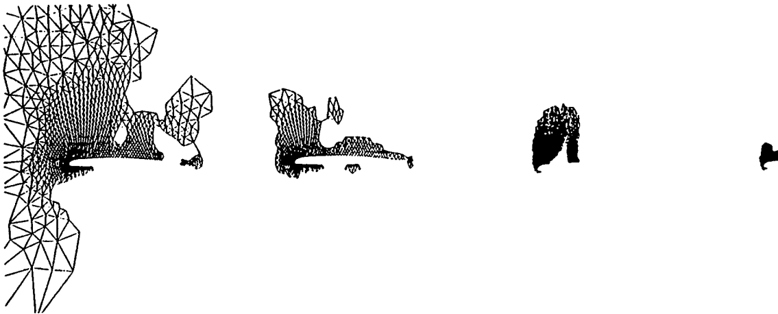
Figure 38: Third and fourth adaptive levels in the zonal fine-grid scheme for computation of flow over tandem airfoil configuration.
