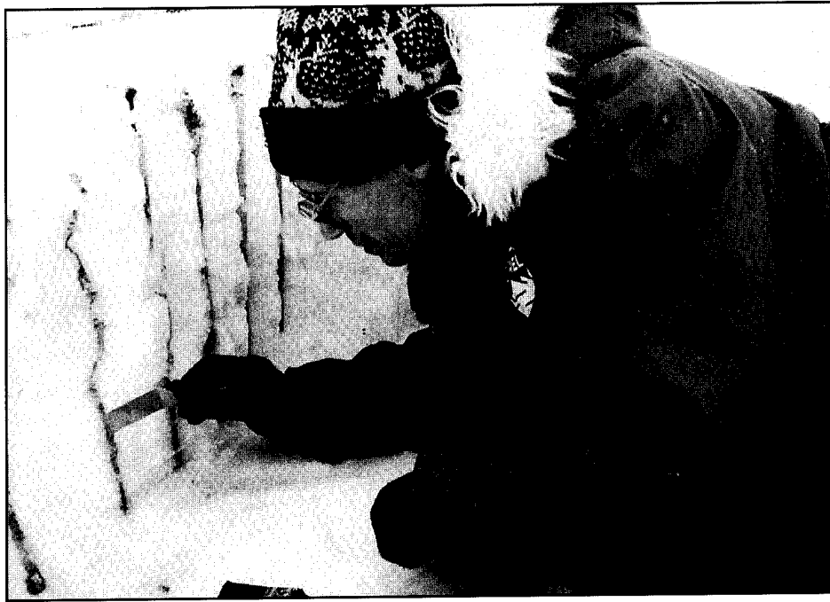
Figure B2. Removing snow to show deformed chalk holes.
