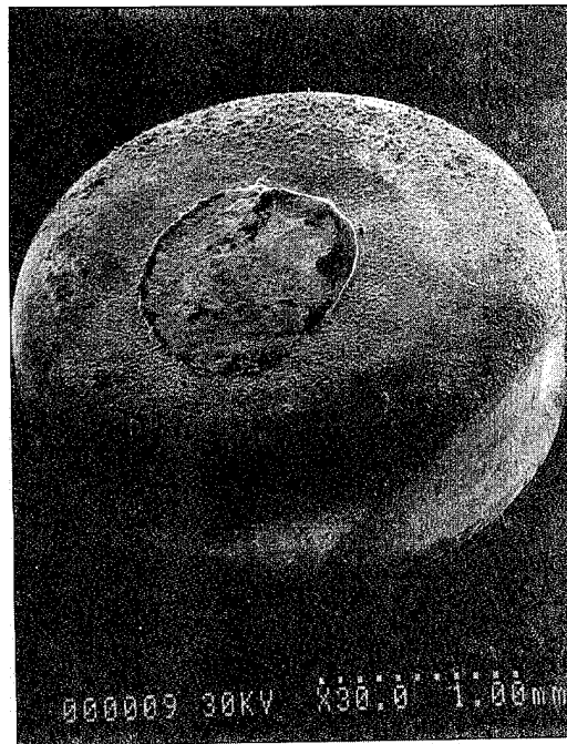
Figure 3.12 Contact from a 10 A circuit breaker cycled 20,000 times at rated ac load current at 120 Vac / 60 Hz. Magnification: 30X.
