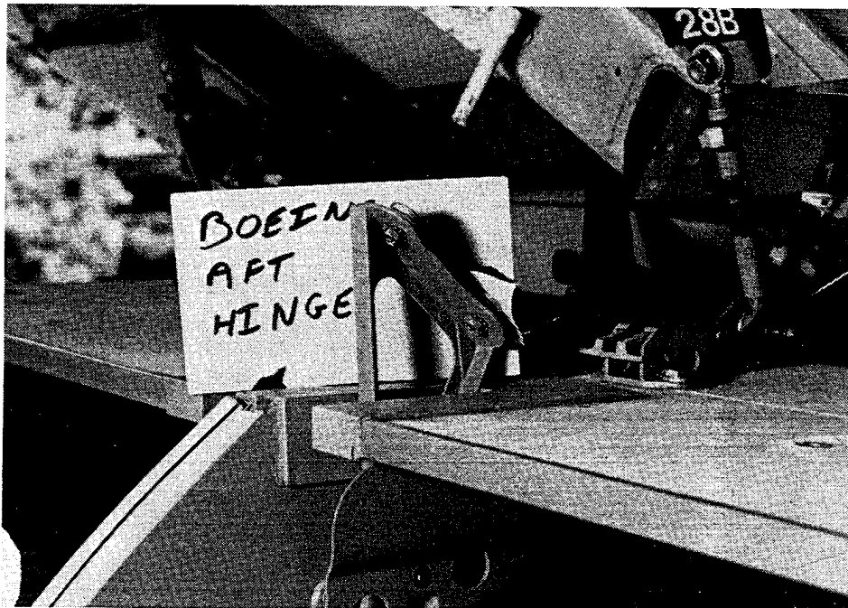
FIGURE 44. BOEING BIN BROKEN AFT HINGE, POSTTEST
