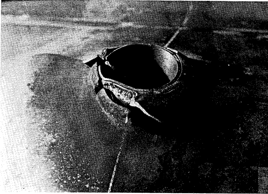
FIGURE 59. AUXILIARY FUEL TANK DRAINAGE HOLE CLOSE UP, POSTTEST
