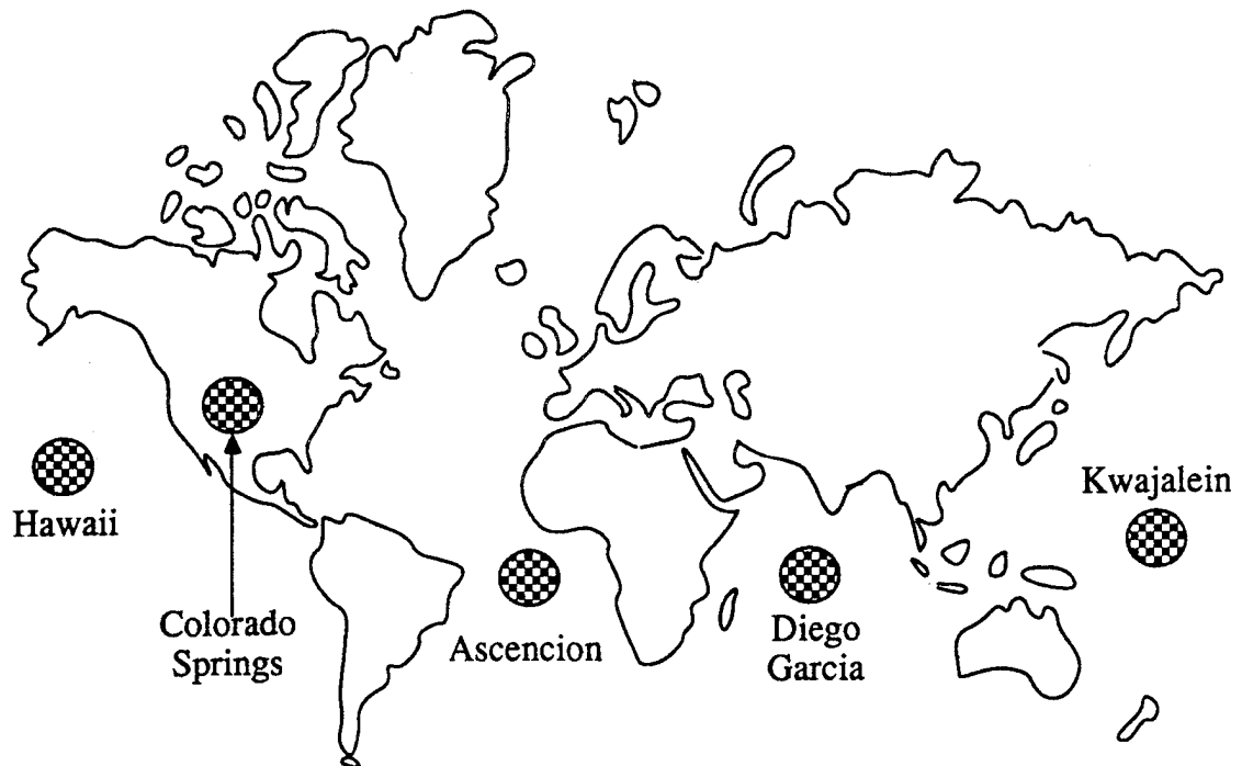
Figure 3.1 GPS Control Stations
