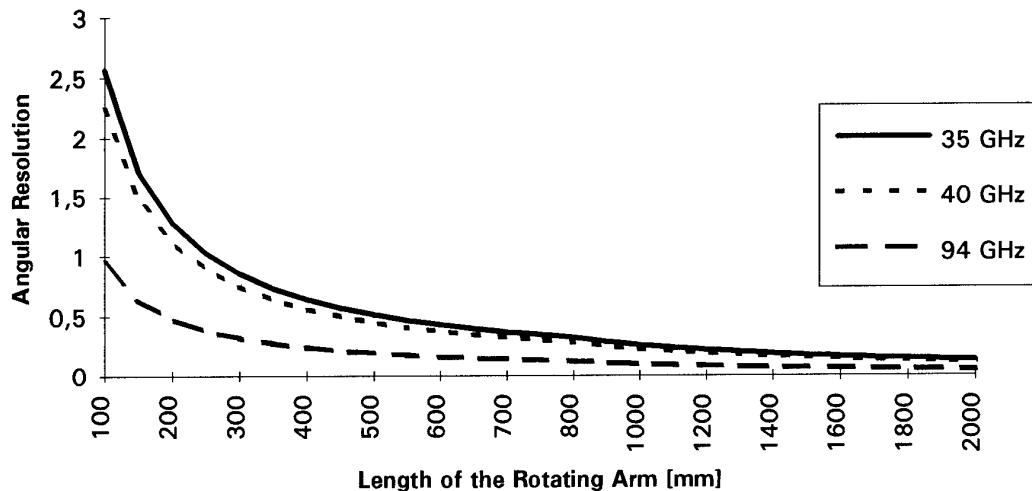
Figure 8: Azimuth Resolution of ROSAR Technology Radars
