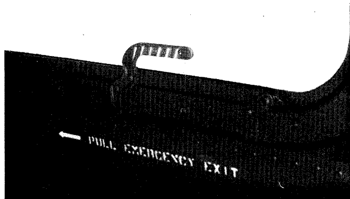
Figure 5. UH-1 cabin emergency egress handles.
