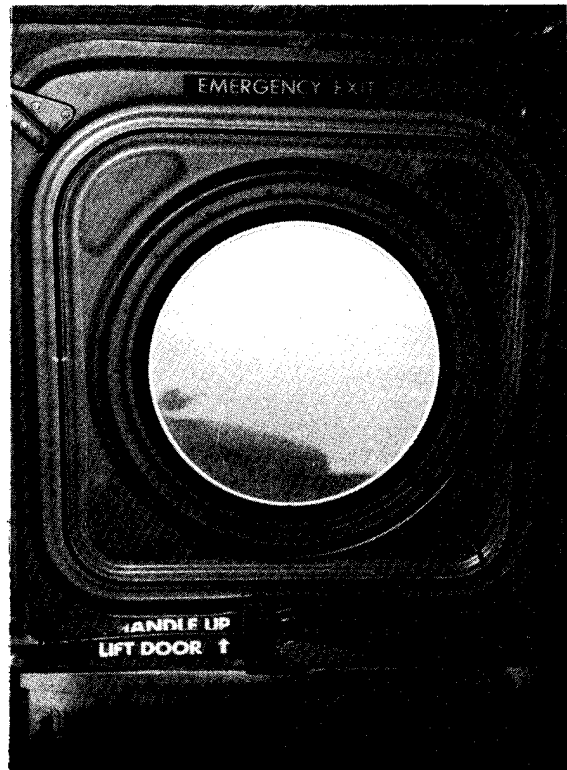
Figure 31. CH-47 cabin area emergency egress door strap.
