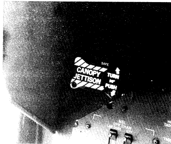
Figure 19. AH-64 copilot/gunner emergency egress handle.
