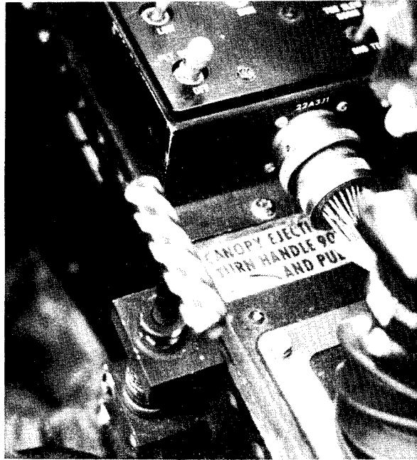
Figure 14. AH-1 copilot/gunner emergency egress handle.
