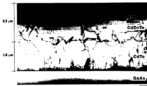
Fig. 9. Cross-sectional TEM of (111) oriented CdTe films on GaAs substrate with misorientation (100) off 2^\circ \rightarrow [110] showing no twins.
