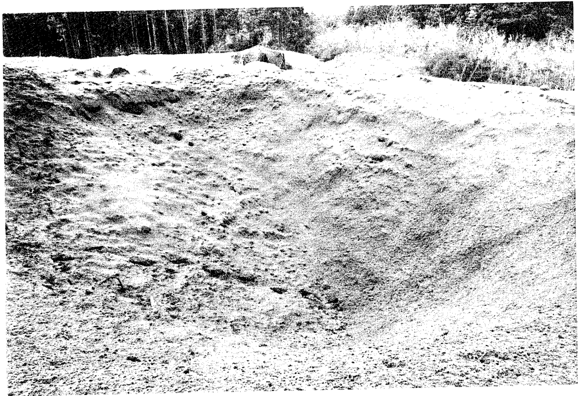
Figure 35. Resultant Crater Approximately 45 Feet in Diameter and 15 Feet Deep
