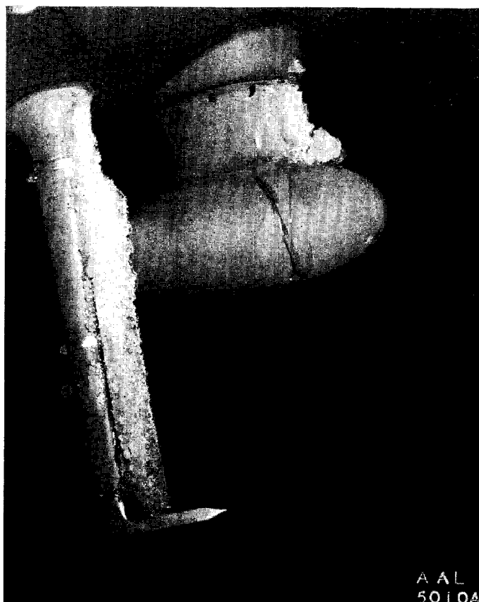
FIGURE 29.—Ice accumulations on the right airspeed mast and loop antenna of the test airplane after flight 29. Photograph taken after landing.
