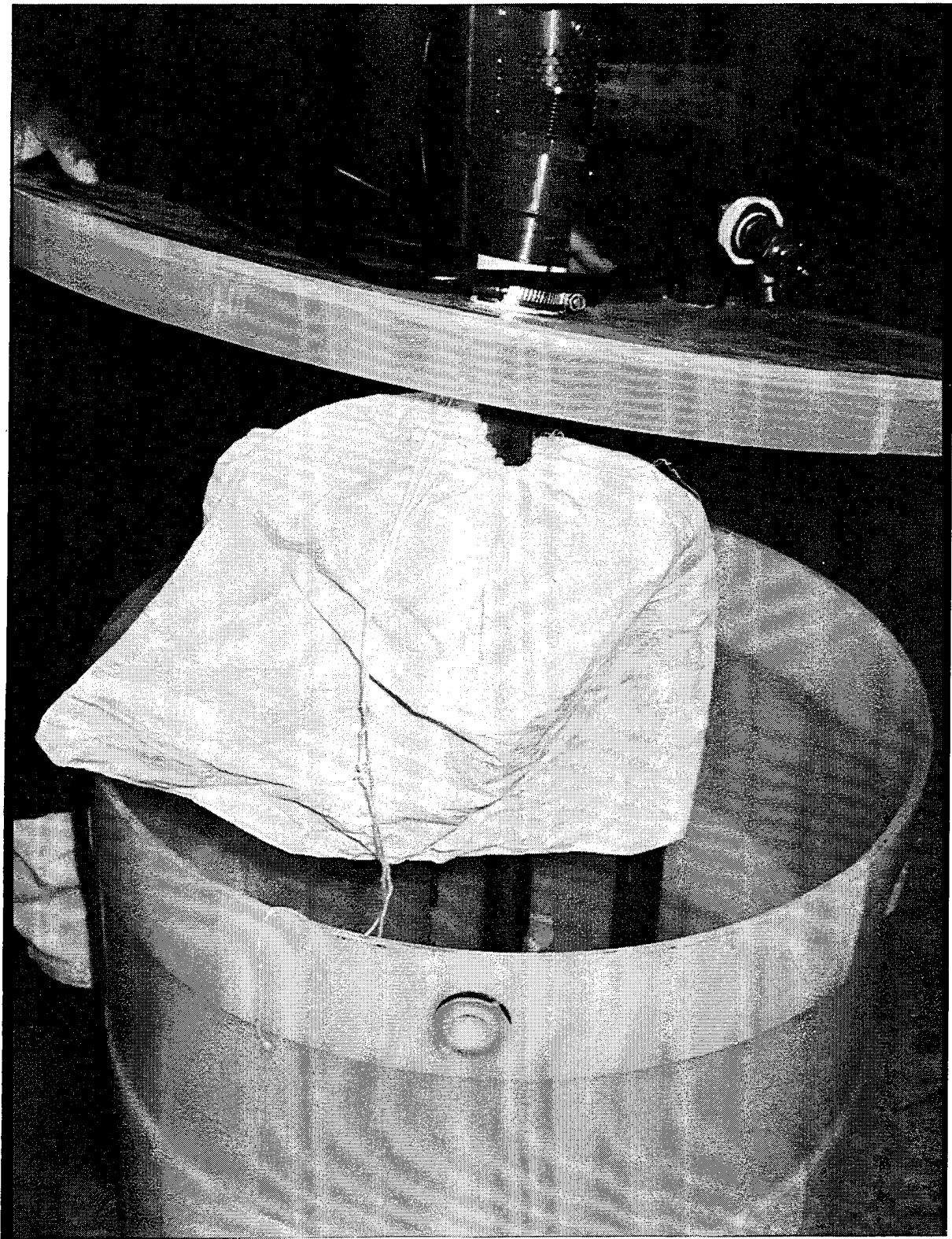
Figure 5. Initial-tank detail showing the prefilter attached.
