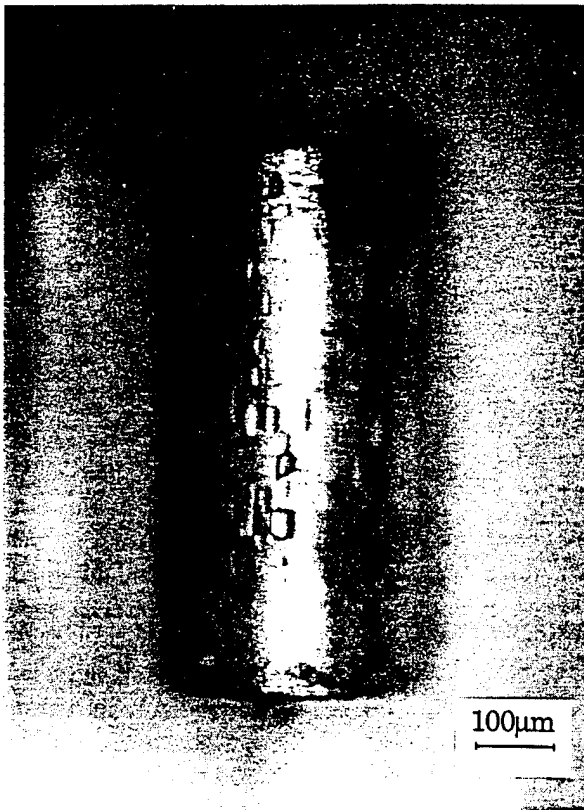
Fig. 9. Dislocation etch pits observed on the outer surface of the SBN61:Ce single crystal fiber.
