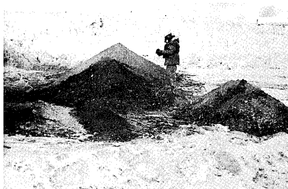
Figure 7. Inspecting DCR-treated soil-like material.
