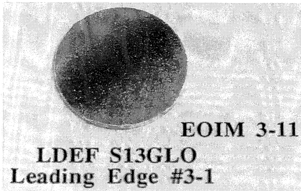
Figure 9. Post-flight photo of EOIM3-3-1, S13GLO LDEF LE (contaminated).
