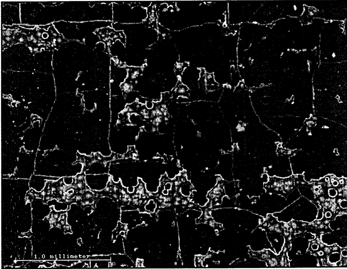
Figure 14. Fluorescent penetrant inspection of the coating crack pattern revealed a generally rectangular crack pattern oriented parallel to the specimen major axes.
