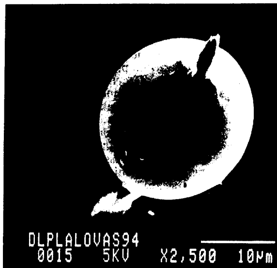
Figure 3. Scanning electron microscopy (SEM) micrograph of lovastatin needle embedded in poly (DL-lactic acid) following RESS coprecipitation from supercritical carbon dioxide. Extraction conditions: 200 bar, 55°C, pre-expansion temperature: 80°C. [Reproduced with permission from ref. 27. Copyright (1993, American Chemical Society)].
