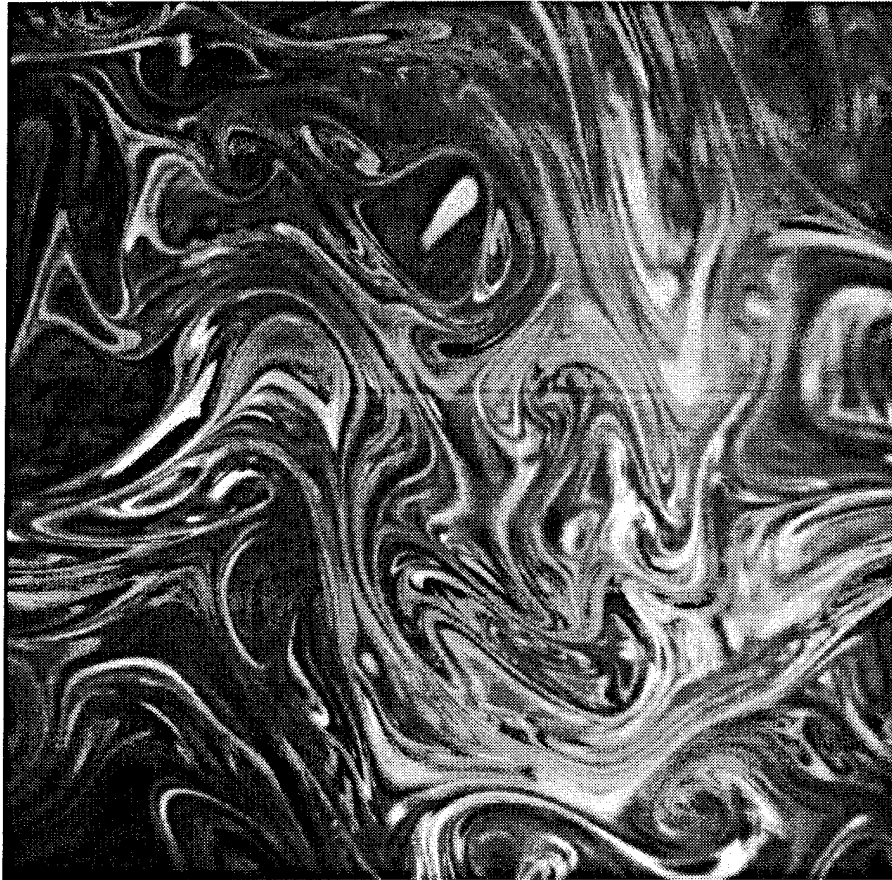
Fig. III.11. Laser-induced fluorescence, 512 \times 512 -image data used for Oseen vortex test case. Data digitized at 11 bits/pixel.
