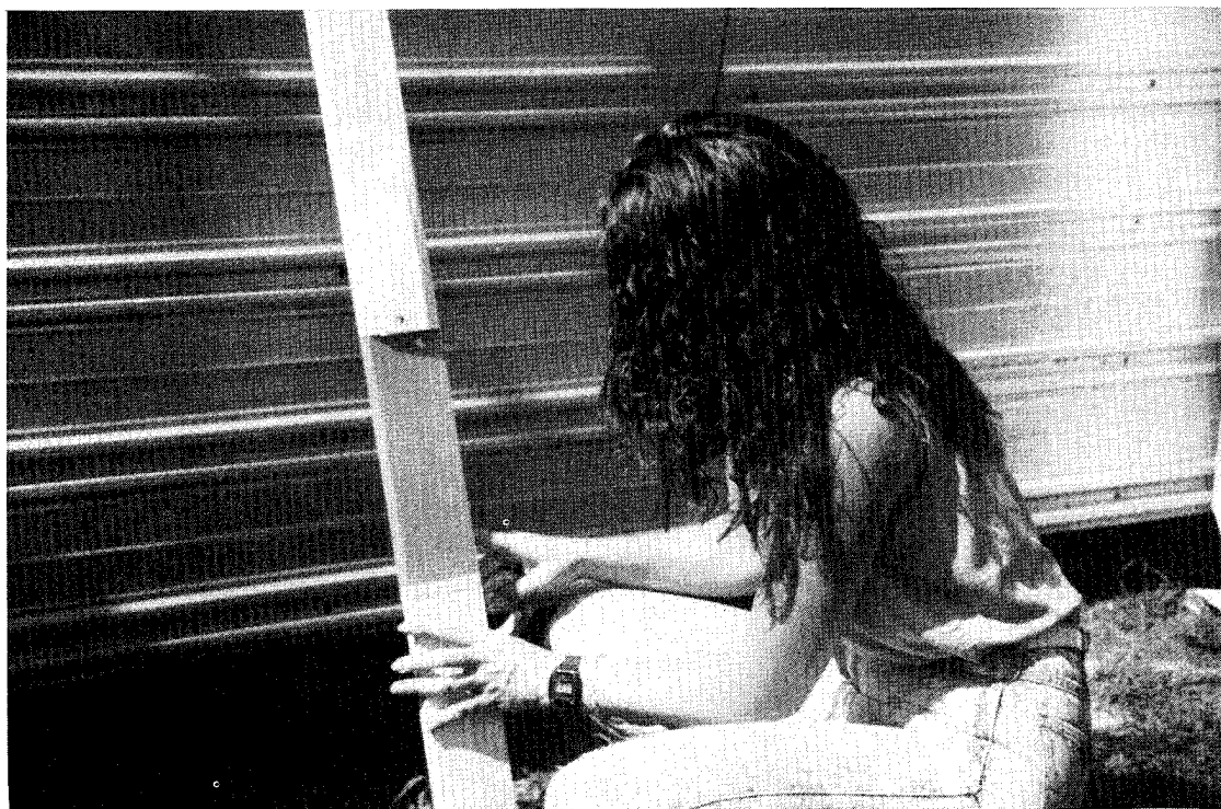
Figure A1. Wrapping alternate sections of the board for painting
