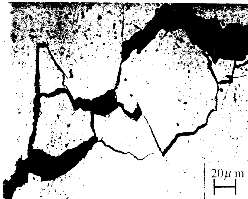
Figure 1.3: a) Opposite faces are "wedged open". b) Fracture surfaces are shattered and distorted due to contact each other.
