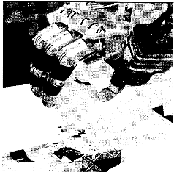
Figure 7: Side view of lightbulb insertion operation, showing binocular eye-in-hand camera configuration.
