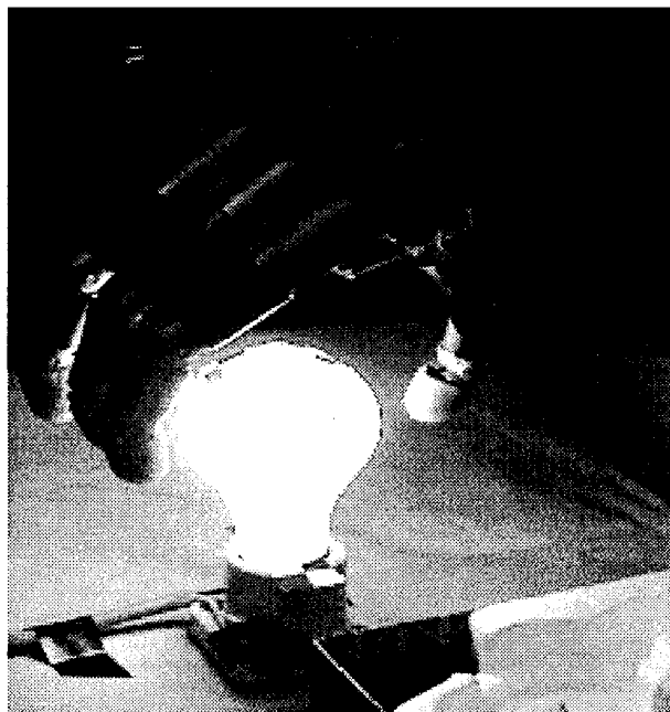
Figure 8: View of lightbulb insertion operation from eye-in-hand camera, showing pre-pickup, pickup, pre-insertion, pre-rotation, and completed phases.
