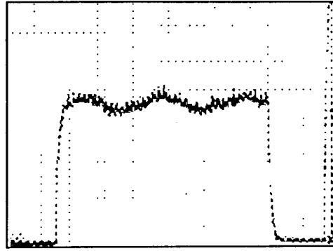
Figure 8. CVSA output when the input is an 8 millivolt peak-to-peak 1000 Hz sine wave modulated at a 10 Hz rate.
