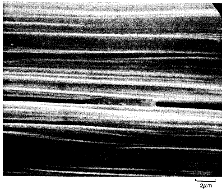
Fig. 18 SEM of Silicon Nitride Coated HTS Graphite Yarn
