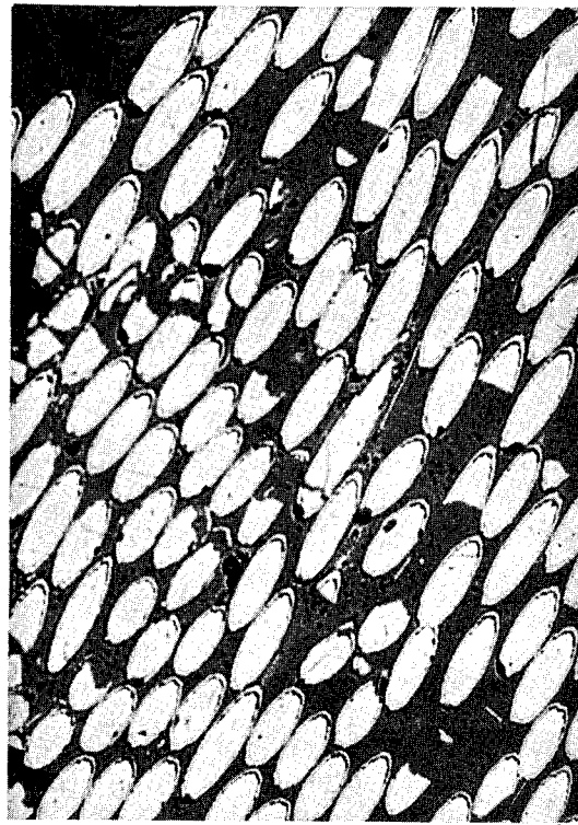
Fig. 22 CVD \text{Si}_3\text{N}_4 Coated HMS Yarn
