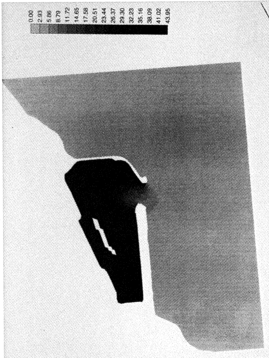
Figure 25. Contour plot of conservative tracer concentration at low tide, 1 day after it was introduced into the existing harbor condition
