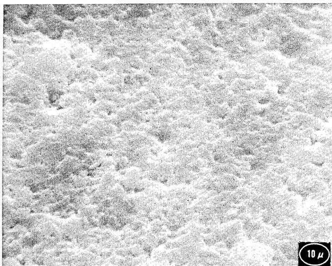
FIG. 6. Texoprint latex-modified natural paper; 1,000X.
