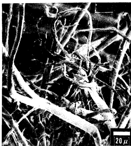
FIG. 7. Composite form of PRD 49-IV after impact with .22 Caliber missile; 360X.
