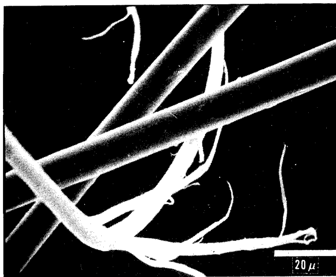
FIG. 6. Fibrillated fiber of PRD 49-IV after slow-speed test; 800X.
