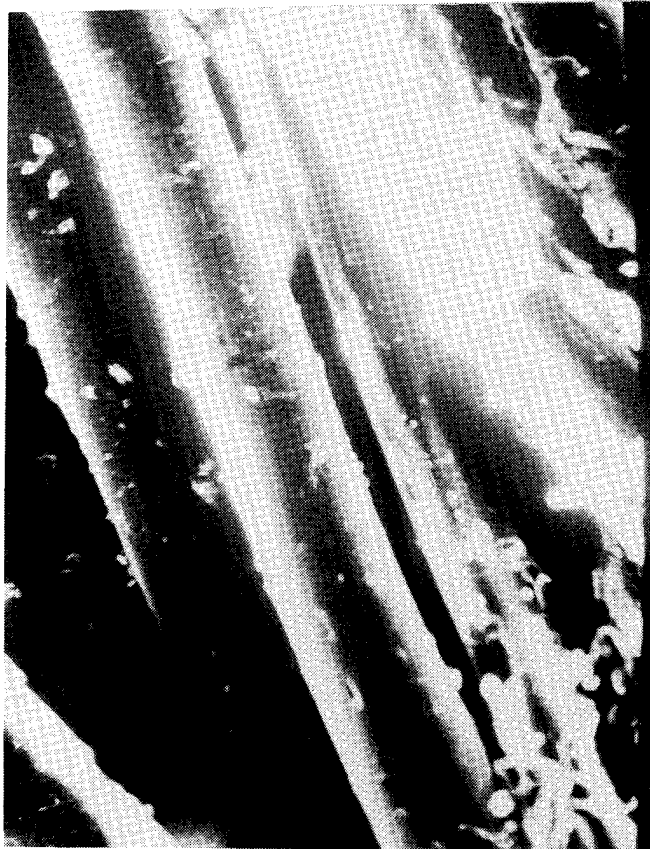
Figure 57. SEM micrograph of a Kevlar fiber within the kink band (1300 X).
