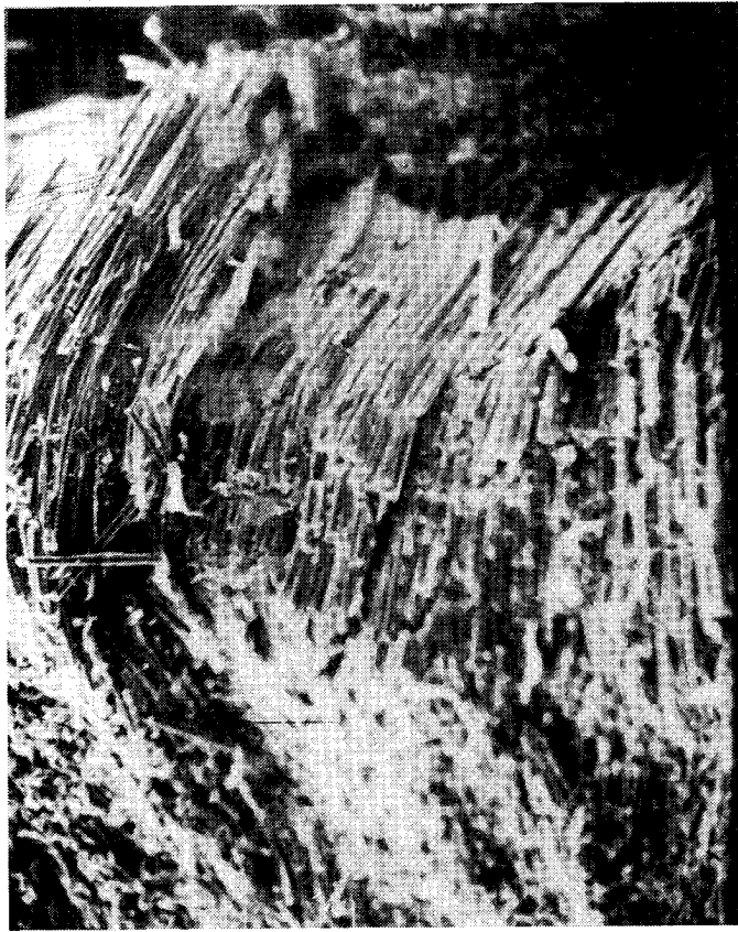
Figure 52. SEM micrograph of the fracture surface of a T300/PPS specimen (125 X).
