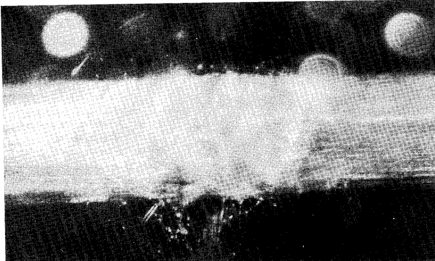
Figure 4. Localized buckling of E-glass bundle in Epon 828/Z (180 X).
