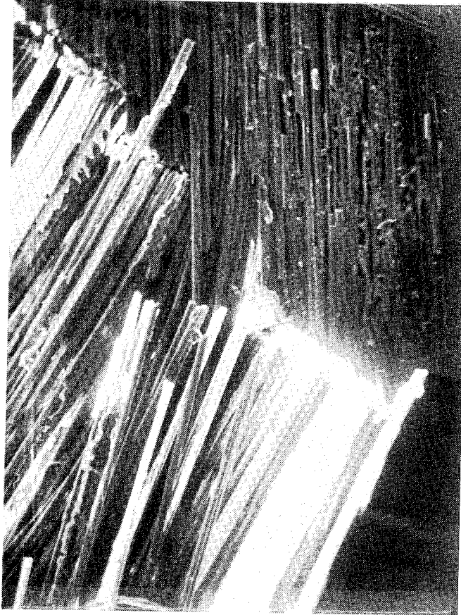
Figure 60. Fiber fractures at the kink band boundary of a S2-glass/epoxy specimen tested at 100 °C (150X).
