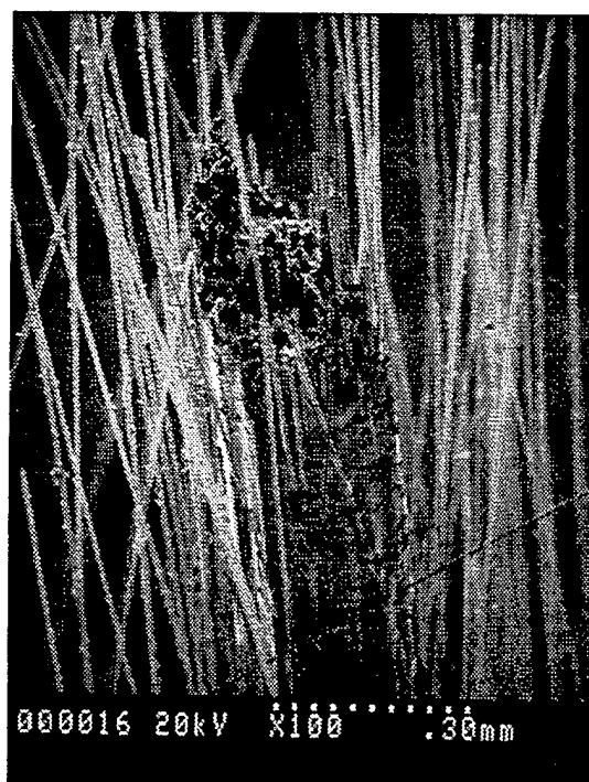
b. Hydrazine exposed T-300/polycyanurate composite
