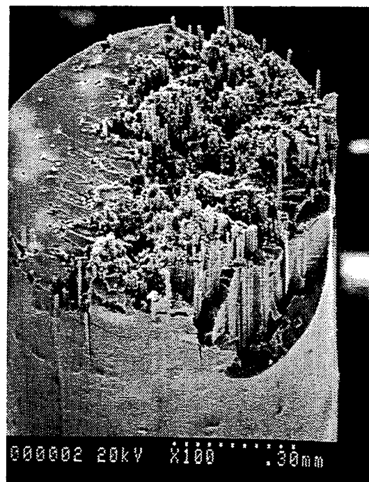
b. Hydrazine exposed T-300/epoxy composite
