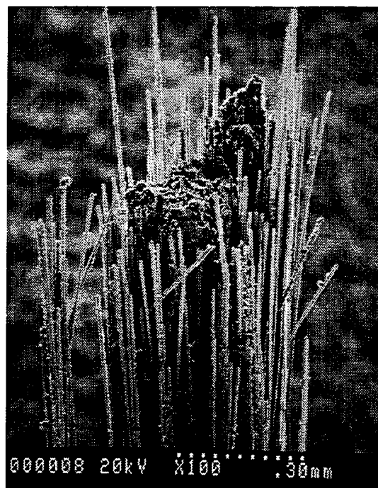
c. NTO exposed T-300/epoxy composite
