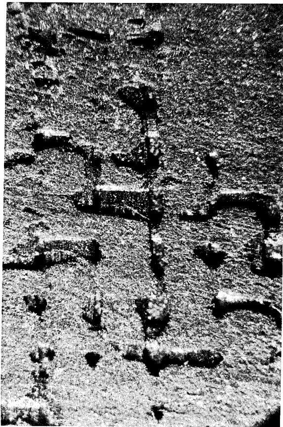
FIGURE 14 PHOTOMICROGRAPHS OF THE FAILED ADHESIVE BOND LINE OF TITANIUM LAP SHEAR SAMPLES BONDED WITH EXPERIMENTAL NR-150 ADHESIVES (20X MAGNIFICATION) SAMPLES TESTED AT R.T.
