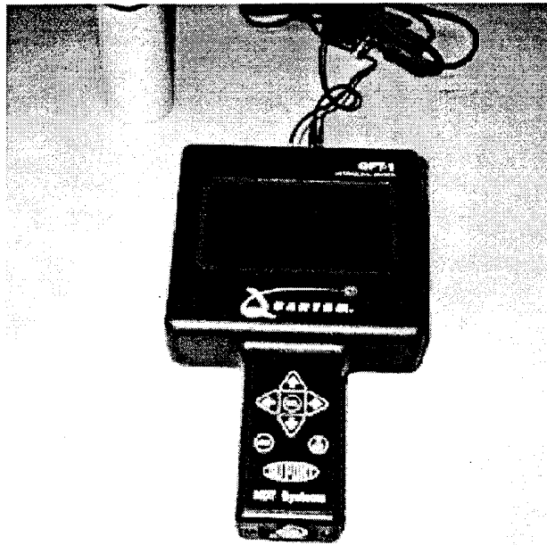
FIGURE 8. ULTRASONIC THICKNESS GAGE USED FOR THIS EXPERIMENT. THIS UNIT IS PORTABLE, AND HAS SETUP STORAGE CAPABILITY. THE UNIT ALSO HAS BOTH THICKNESS READOUT AND AN A-SCAN PRESENTATION DISPLAY.
