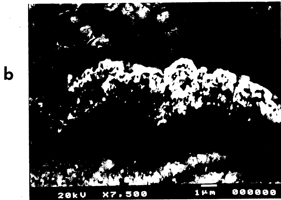
Figure 24. SEM image of the heat treated six layer Ir-Al coating showing (a) delamination, and (b) buckling.
