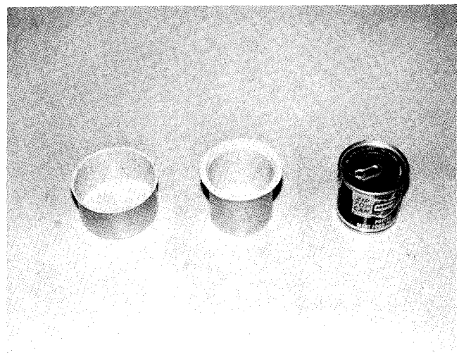
FIGURE 6: Deep-Draw Stages of Container Manufacturing
