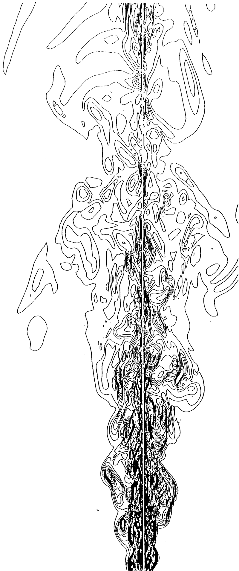
Figure 1: LES simulation of a turbulent round jet at Re = 15,000 without SGS model c_s = 0.0 : Vorticity magnitude at time t = 898 .
