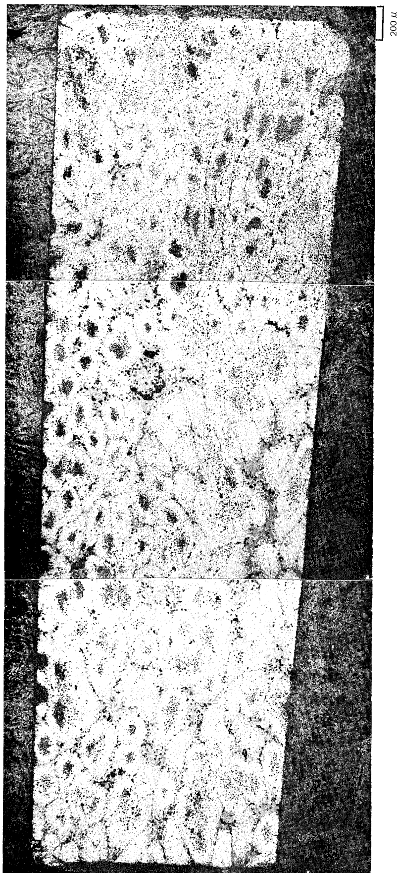
TAPE-MAP OF UNFRACTURED SAMPLE LB96 CELANESE DG-102 FIBER, 7740 GLASS MATRIX, HOT PRESSED AT 1075 °C
