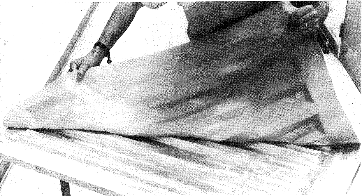
Figure 20. Rubber Bag Being Removed from Mold
