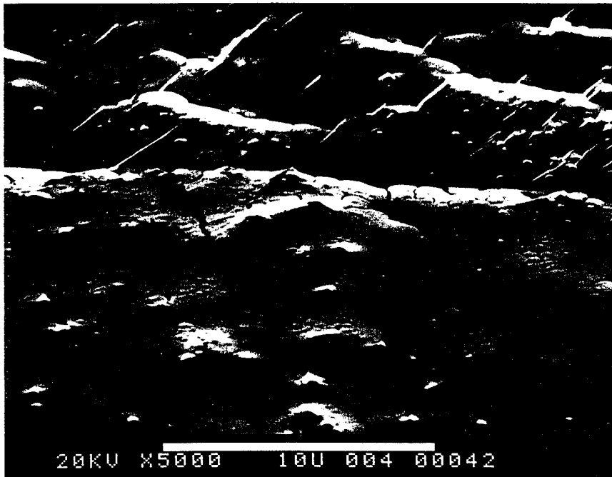
Figure 5 Carbon surface layer after long duration low rate C + implant
