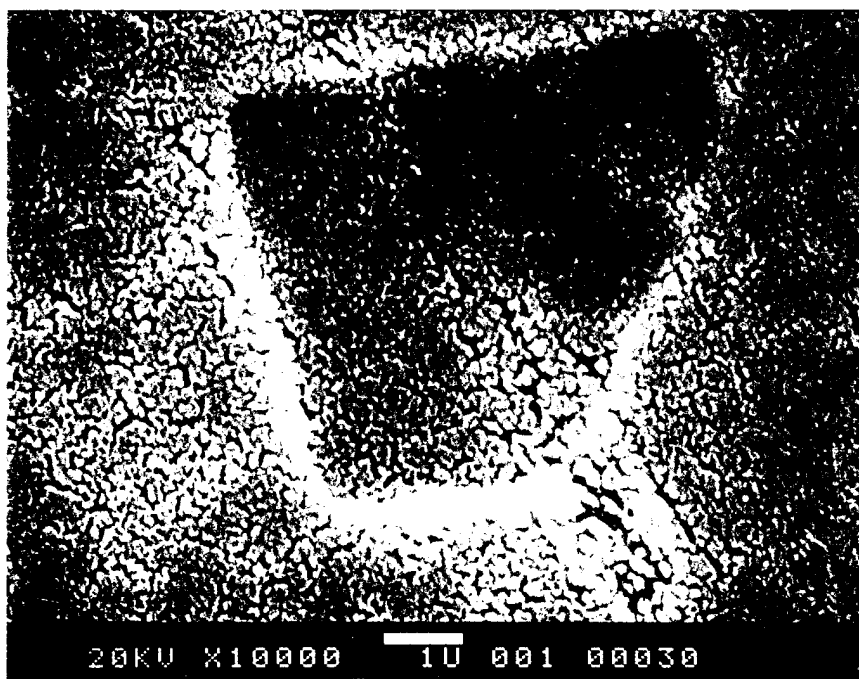
Figure 16 Outline of oriented cavity covered by coating after H 2 + and C + implants
