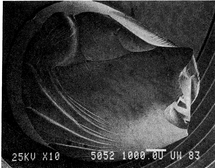
Figure D22. Fibredux 914 Neat Epoxy Torsional Shear, 23°C, Dry.
