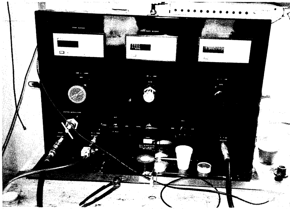
Figure 108. Calibration unit employing digital pressure gages.
