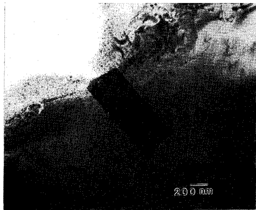
Fig. 5. Precipitation of \text{MgAl}_2\text{O}_4 , away from the interface, after annealing at 680°C for 10 h. This spinel, along with some \text{Al}_2\text{O}_3 were the only precipitates observed. Usually, these were found not to adhere to the interface.
