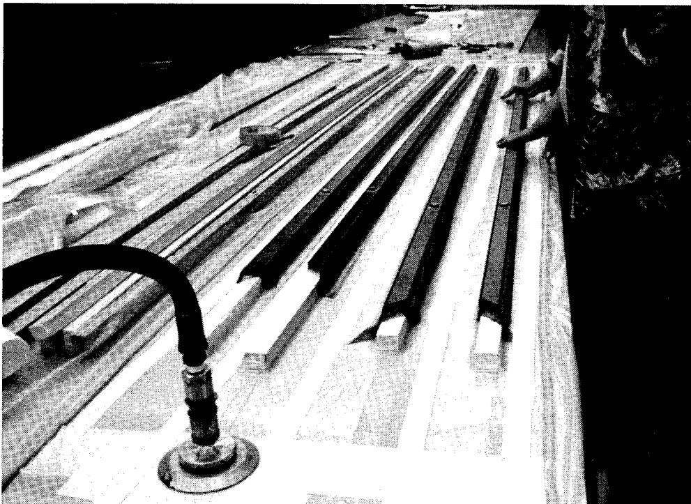
Figure 43. Stub Box I-Stiffened Skin Panel—Layup of I-Stiffeners
