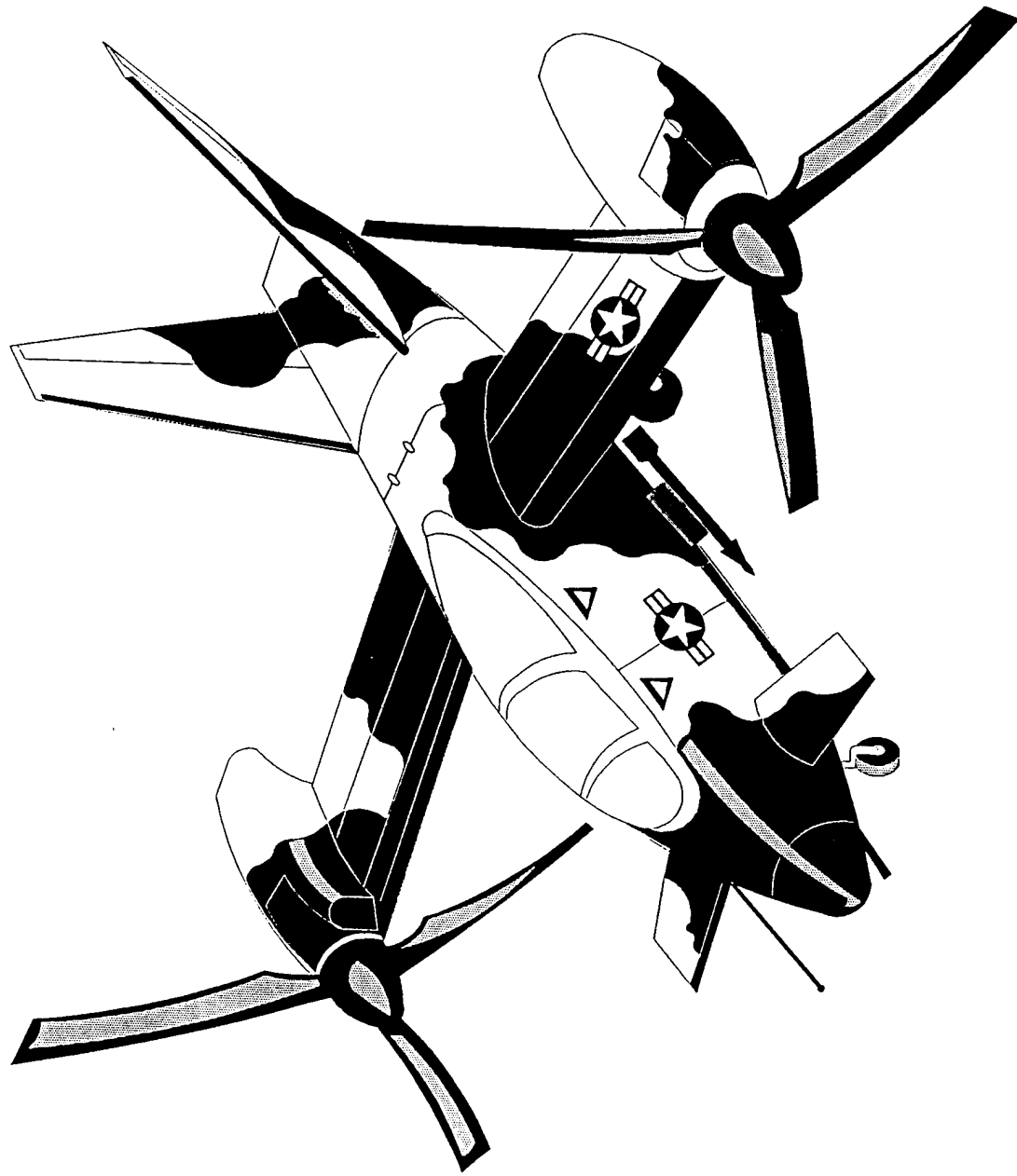
FIGURE 1: Tactical Tilt Rotor Proposed by Boeing Helicopter Company as FAAV Candidate for ART.
