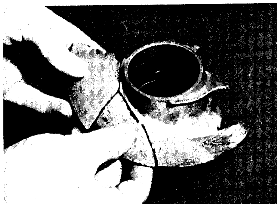
FIGURE VI-44.—Inducer blade failure.
