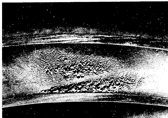
FIGURE VI-36.—Pump blade cavitation damage.
