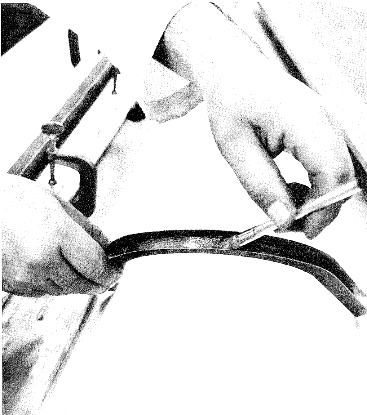
Figure 38. Primer Being Applied to the Inner Section of "U" Channel
