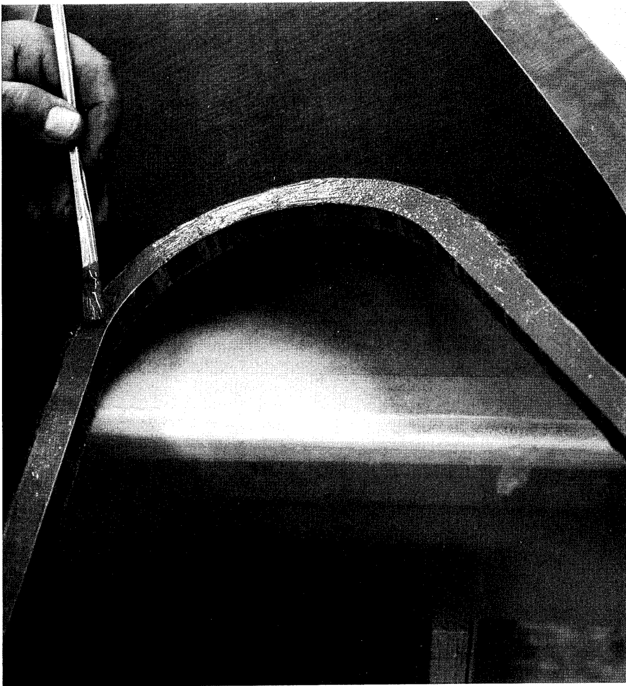
Figure 37. Primer Being Applied on Rib Web For Bonding "U" Channel
