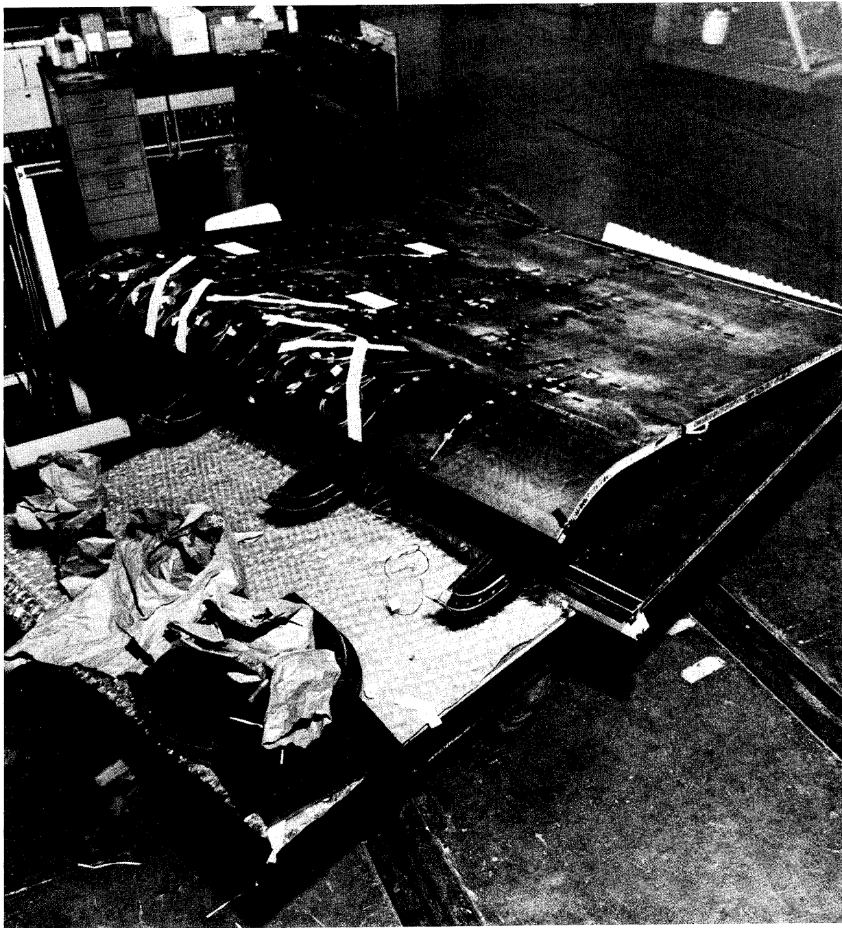
Figure 3-10. Strain Gage, Thermocouples, and Deflection Mounting Tabs - Lower Honeycomb Cover Panel
