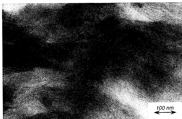
Fig. 3. TEM of the section of molded NCH-15.
