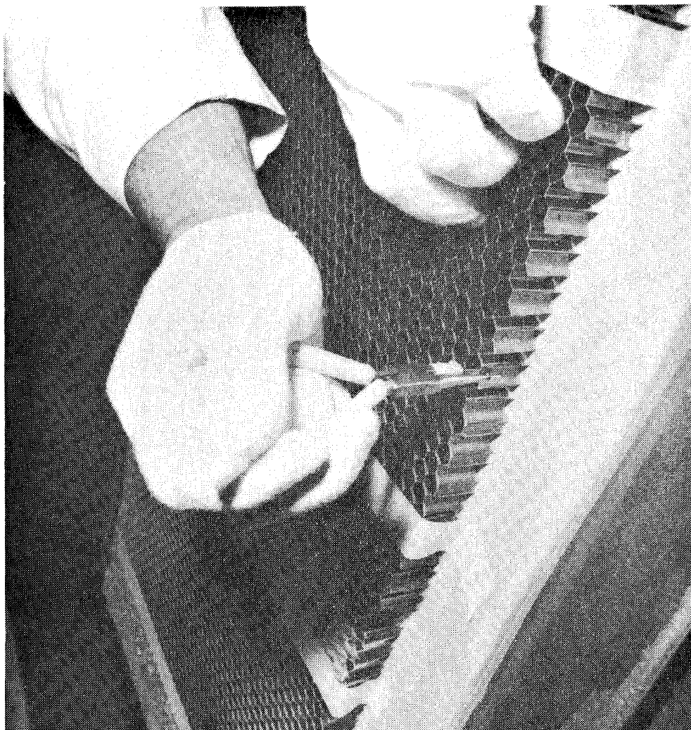
Figure 36.- Perforating honeycomb core at cell node points.
