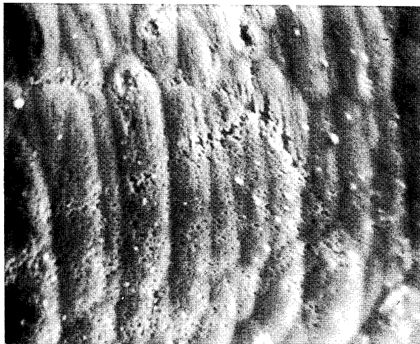
Figure 1. Surface of boron fibers (X2900) in initial state (a) and with signs of borides formed due to interaction with matrix (b, c)
