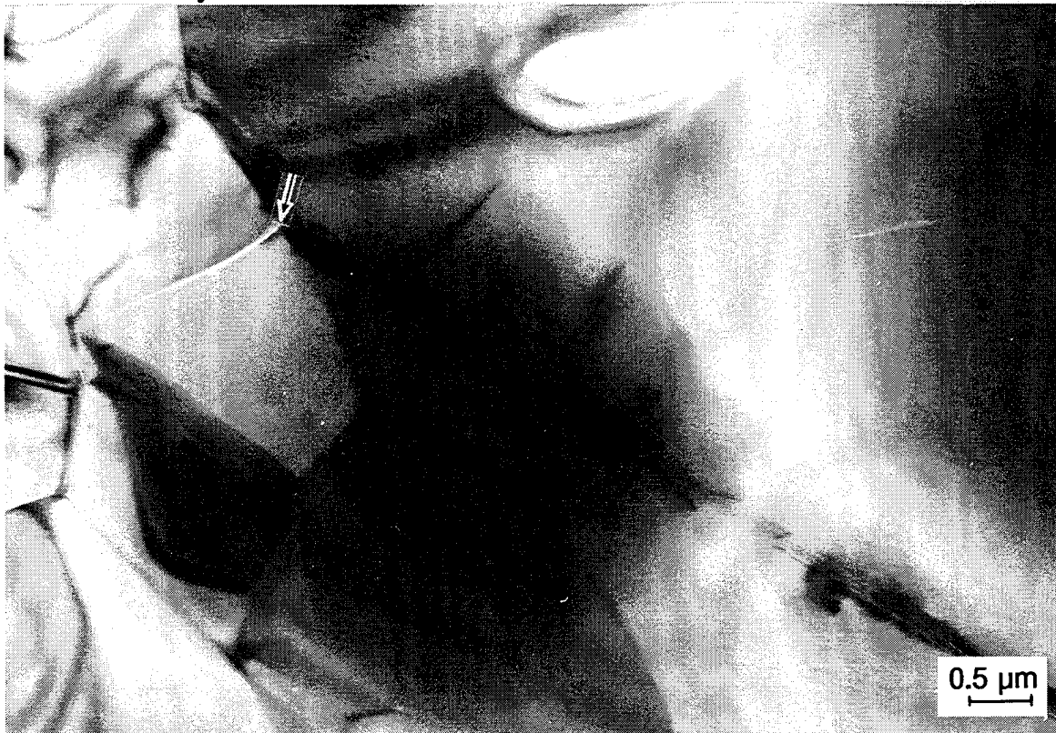
Figure 57. Dislocation slip band (arrow) nucleating transgranular microcrack in adjacent grain.
