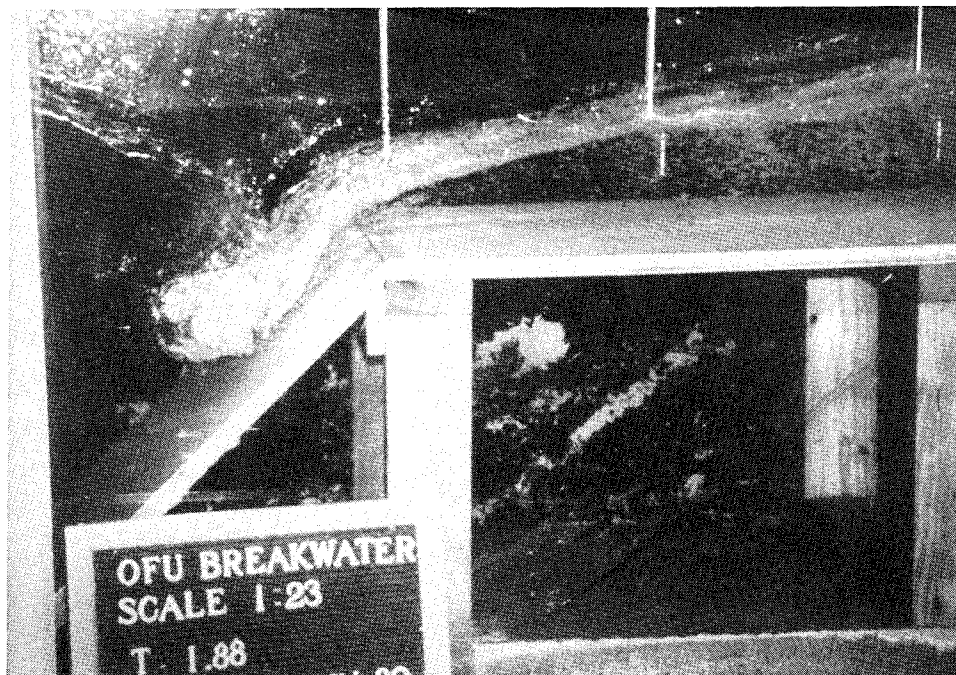
Figure A2. Trough of short-period wave ( T = 9 sec) passing over reef
