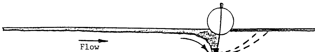
Drainage Due to Excess Oil and Velocity
